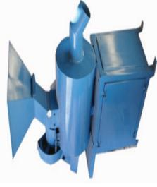
PALM CANNEL BLOWER<br>CAPACITY:300 KG /<br>HR.POWER:<br>MOTOR/ENGINE HP 5.5                                 | 0.9 mill          | SIDO MBEYA |
