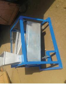
DISTONER MACHINE<br><br>Power 2 HP; 3 PHASE/SINGLE<br>CAPACITY 800 kg/hr.<br><br>POWER 4Hp, 3 PHASE /<br>SINGLE<br><br>CAPACITY: 1.5 tons/hr | 2.5 mill<br><br>4 mill    | SIDO MBEYA |
