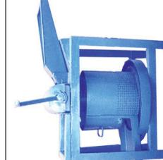
PALM OIL PROCESSOR<br>CAPACITY: 240 KG/HR<br>POWER: 5 HP, 3 PHASE MOTOR                                      | 3.5 mill              | SIDO MBEYA |
