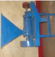
MAIZE HULLER<br>POWER: 15 HP, 3 PHASE<br>MOTOR; 13 HP DIESEL<br>ENGINE SPEED: 1000 RPM<br>CAPACITY : 300-350 KG/HR         | 2.7 mill | SIDO KIGOMA |
