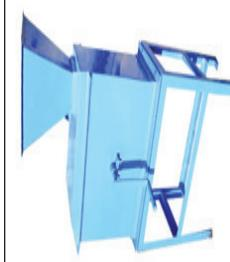
GROUNDNUTS SHELLER<br>CAPACITY: 15 KG/HR<br>POWER: MANUAL<br>5.5 hp                                                                                     | 0.68 mill<br>2.2 mill | SIDO MBEYA |
